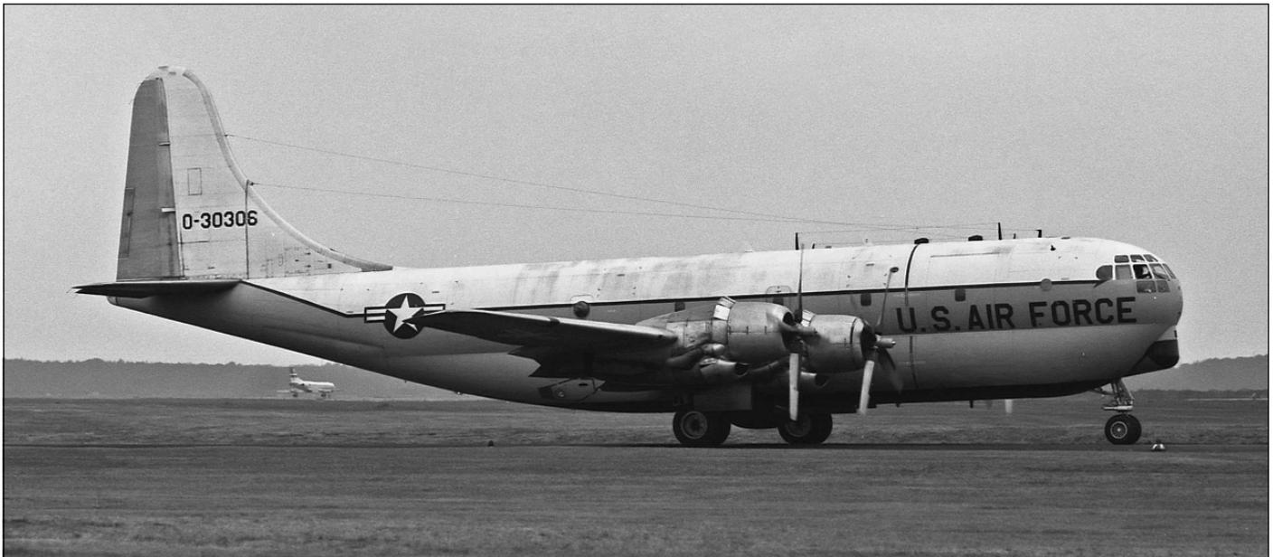
7405th SS used a fleet of C-97Gs, with 53-0306 illustrated here. The aircraft's reconnaissance equipment, a 48" oblique and a 12-inch vertical camera, is hidden from view by several large panels which could be opened during flight, but closed again before landing. One of these panels is located in the fuselage just in front of the engines. (Rhein-Main late 1960s, Peter Zastrow)
