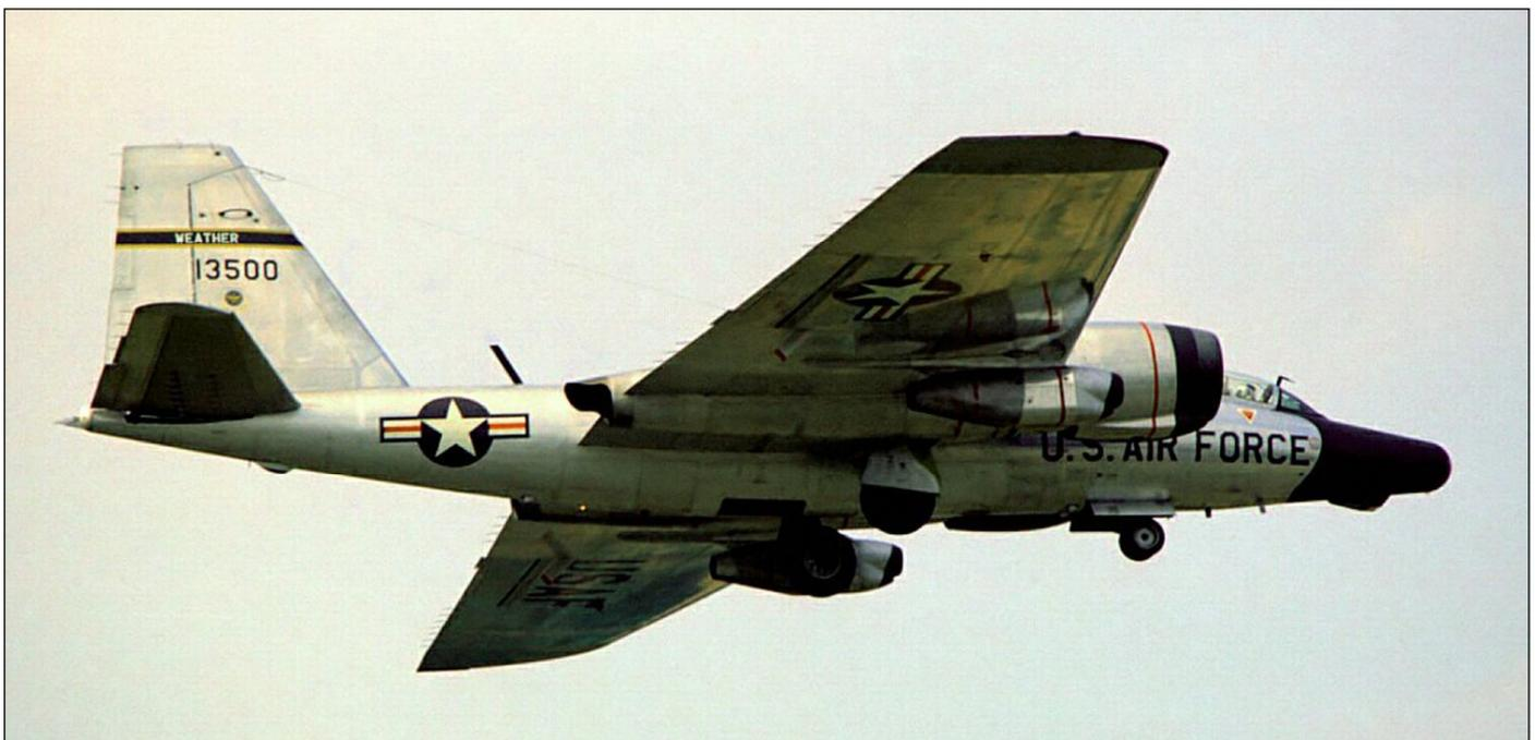
RB-57F 63-13500 seen on final approach to Rhein-Main. Note that this is a four-engine B-57; it has two additional jet engine pods under the wings. (Manfred Faber)
