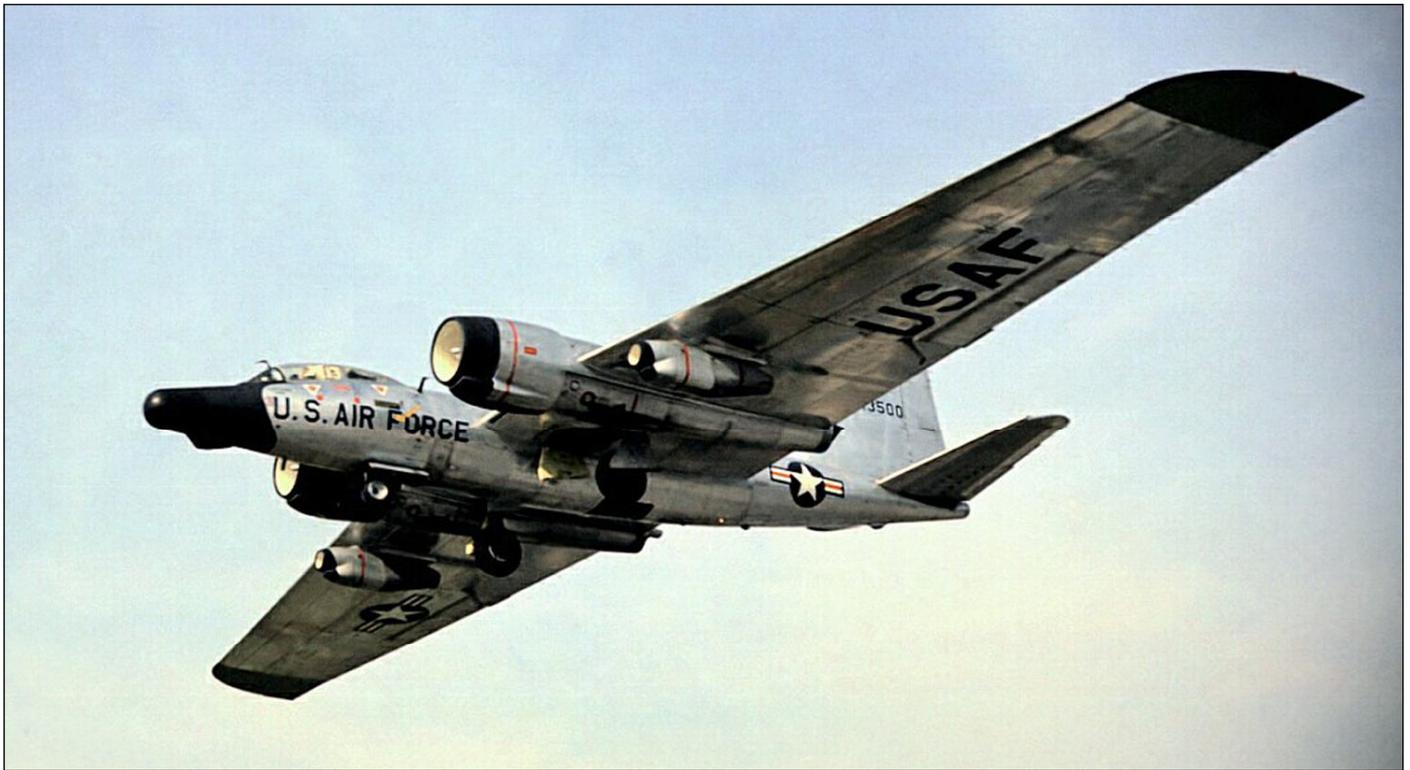
*The impressive wing of 63-13500 is the most distinctive feature of the RB-57F, but other apparent changes are the different engines, TF33s - compare with the other B-57 photographs on previous pages. Also noted the podded engines just outside of the nacelles. The shot was taken at Rhein-Main. (Manfred Faber)*
