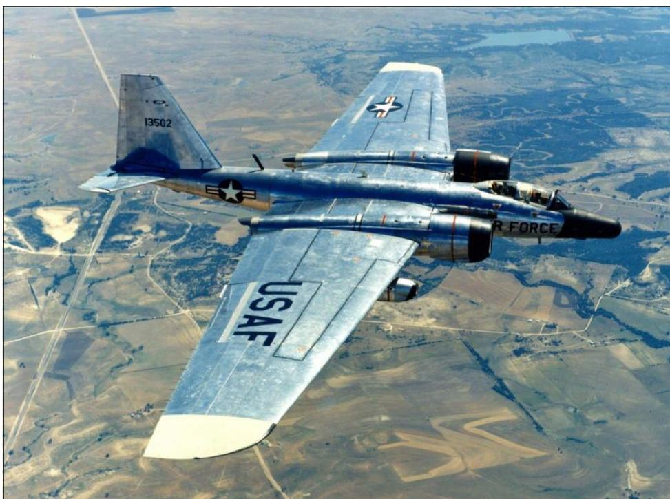
The RB-57Fs were awesome machines with an incredible wingspan of 122ft, as shown in this shot of 63-13502, somewhere over the USA. They were nothing like the original RAF Canberra! The aircraft served with 7407th SS in 1966. (USAF photo via Henk Scharringa)
