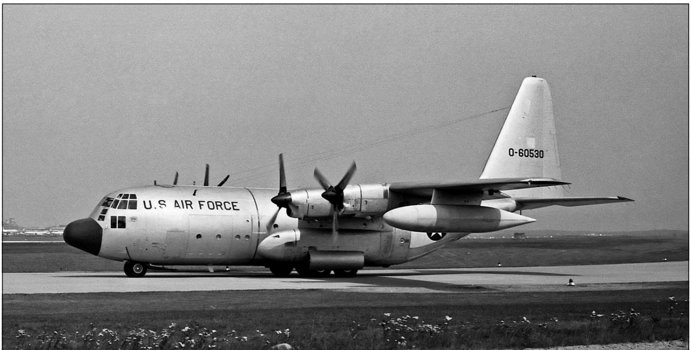
*C-130A-II 56-0530 on the taxiway at Rhein-Main in 1970. There were few features to distinguish the aircraft from normal cargo C-130s, apart from the lack of camouflage and the presence of the enlarged pod under the wing, which contained some of the aircraft's sensors and equipment.*
