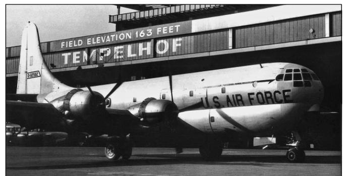
C-97A 49-2592 at Tempelhof Airport, Berlin, in the mid-1950s. With code name 'Pie Face', this aircraft was the first specially-modified reconnaissance aircraft supplied to 7499th SS, arriving in 1953. It carried a special 240-inch focal length camera. Like most of its C-97 successors, it had an open cargo deck, with its special equipment hidden below the deck and in the crew area. (7499th Group Association)
